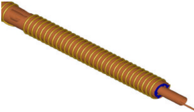
Figure 7: Beam-screen / cold-bore assembly.
