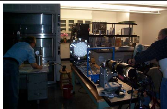
Figure 2: Photogrammetry setup at NIU with projector in foreground, camera on right, projected dots on window, and stationary targets on flange
