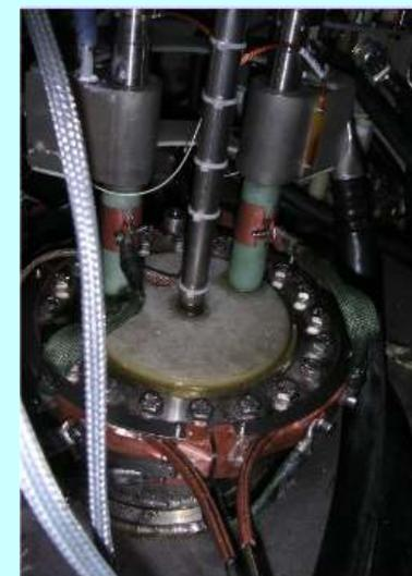
Very difficult access to permit the electrical feed-boxes consolidation with high risk of damage to delicate wiring
