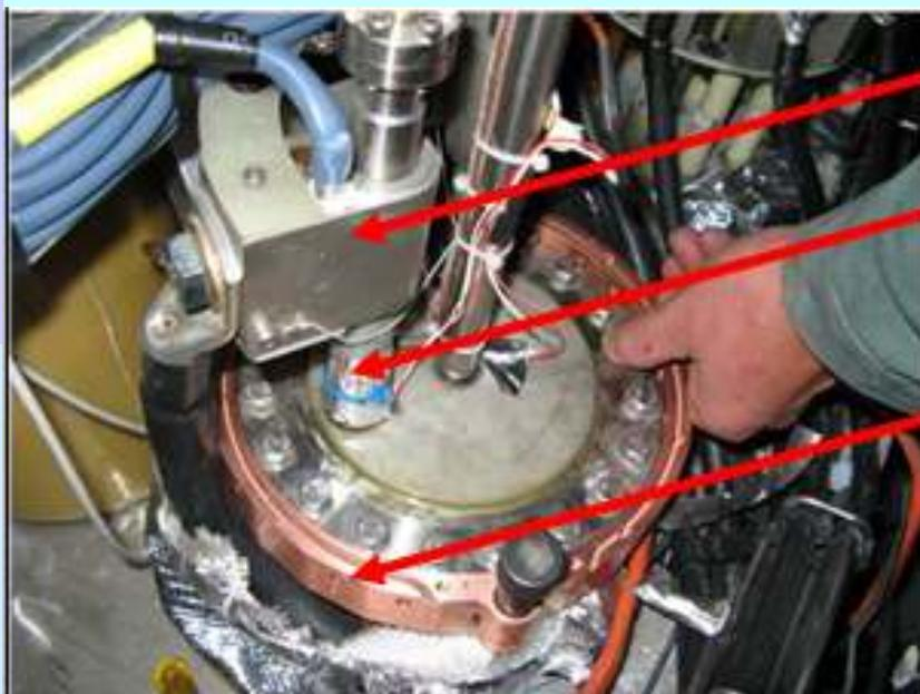
Local heater used to warm up helium gas to room temperature before it is collected in the WRL.
